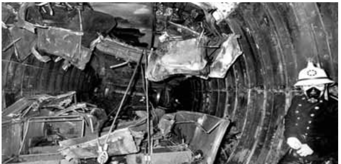
DISASTER: Squashed against the roof of the Tube tunnel at Moorgate is the first coach of the train that smashed into the tunnel wall. Amid the wreckage are the front bogie wheels from the second coach. The foul air forces the fireman to wear a breathing mask.
