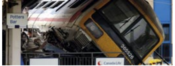
DISASTER: The Health and Safety Executive (HSE) report into the Potters Bar crash released a year later found that the points were poorly maintained and that this was the cause of the accident. Rail contractor Jarvis had claimed that the points' poor condition was due to sabotage but the HSE report found that other sets of points in the Potters Bar area showed similar maintenance deficiencies and the poor state of maintenance "probably arose from a failure to understand fully the design and safety requirements".
